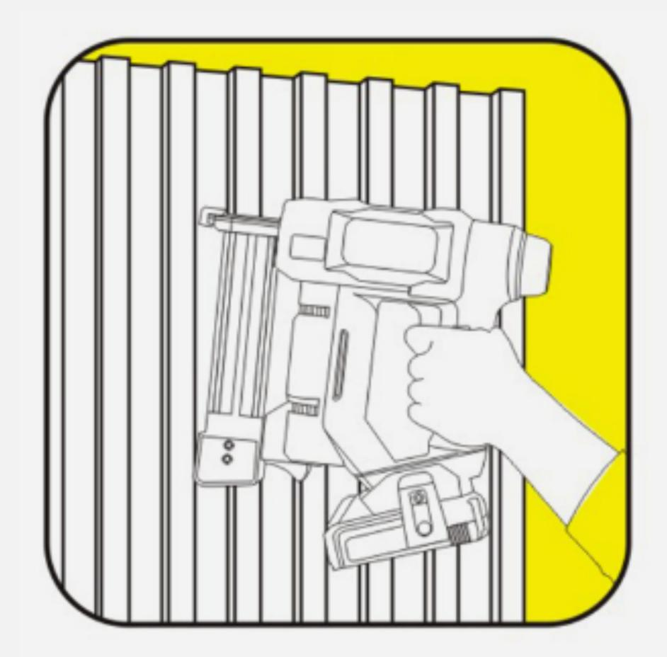
Simply use a pneumatic nailer on the concave part to secure the panels or use the screws provided in the box.
